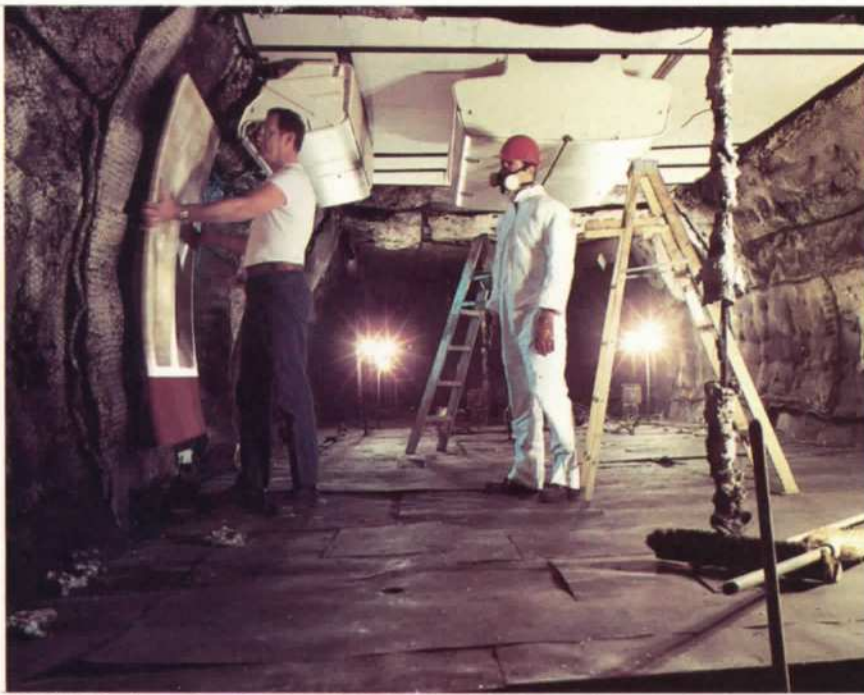
ABOVE: The burned-out interior of a C-133 is rebuilt for use in fire testing by engineering technician Jim Leach, left, and Chris Young. They will reconstruct the plane down to the carpets—and then burn it to a cinder in less than six minutes. BELOW: Inside a wind tunnel sits a de-winged plane, used to test in-flight firefighting methods.
